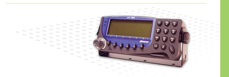
The @Road *i*DT 3000 is an in-vehicle messaging device, used together with @Road GeoManager<sub>SM</sub> *i*LM<sup>®</sup> Mobile Resource Management software. The *i*DT (Internet Data Terminal<sup>TM</sup>) works in conjunction with the GeoManager Messaging and Forms optional feature to provide two-way communication between mobile workers and their dispatchers and managers.
